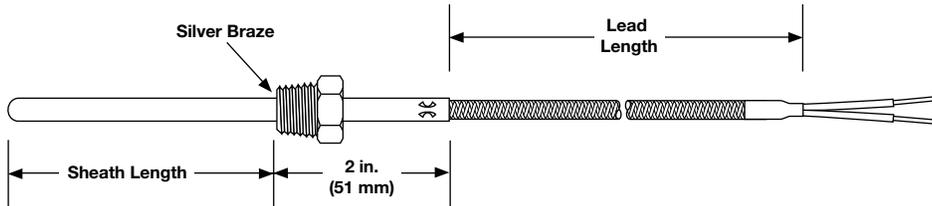
Rigid sheath with threaded fitting provides accurate placement in process applications.
